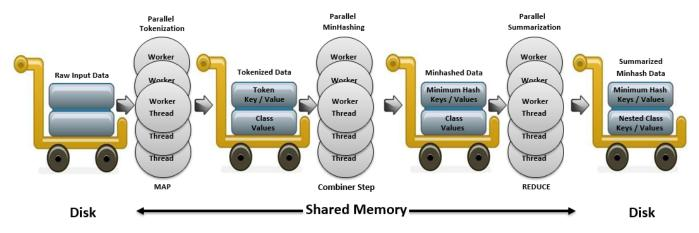
Fig. 1. Strand Map Reduction Aggregation Processing for a Single Training or Classification Worker Process.
